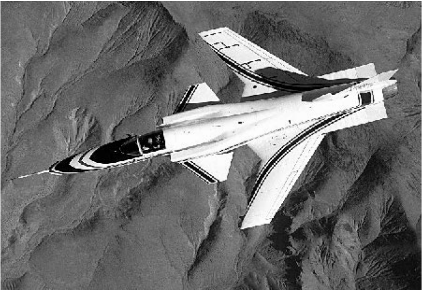
Figure 5.3 NASA-Grumman forward-swept wing, X-29 aircraft. (Courtesy of Dryden Flight Research Center)
